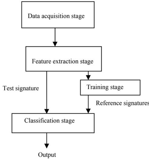
Fig.1. Proposed on-line signature verification system block diagram.
