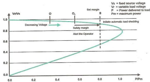
Figure 1: Progress of a voltage collapse case.
