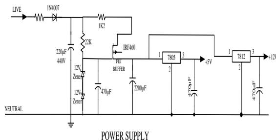
Figure 2 Circuit diagram of the 12V and 5V dc power supply unit
