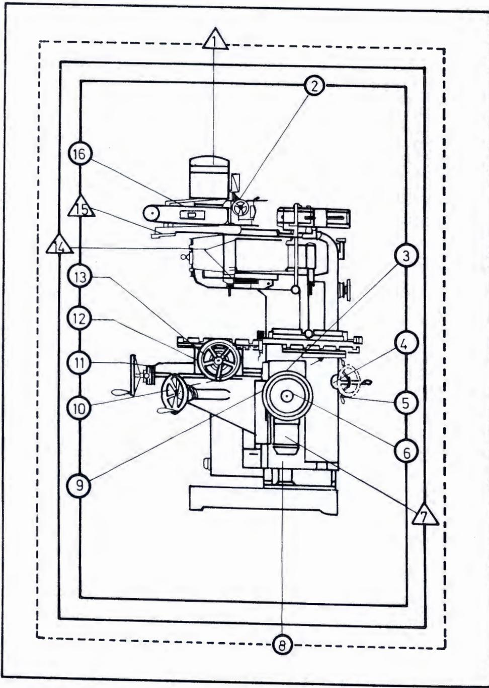
FIG .3 A LUBRICATION DIAGRAM IN WHICH THE FRAMES REFER TO DIFERENT PERIODS OF SERVICE AND THE CIRCLES AND TRIANGLES TO THE TYPE OF SERVICE ( REF.14 ).
