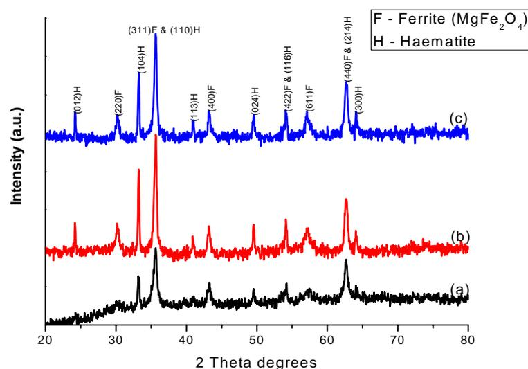
**Fig. 3.** XRD patterns of  $\text{MgFe}_2\text{O}_4$  sample annealed at  $600^\circ\text{C}$  for 2h: (a)  $\text{MgFe}_2\text{O}_4$ -II (b)  $\text{MgFe}_2\text{O}_4$ -III (c)  $\text{MgFe}_2\text{O}_4$ -I.
