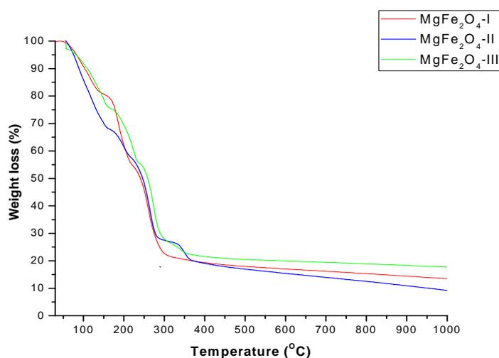
Fig. 1. TGA curves of the precursors gels for MgFe<sub>2</sub>O<sub>4</sub> I-III samples.
