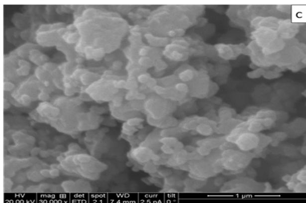
**Fig. 5.** SEM micrographs of  $\text{MgFe}_2\text{O}_4$  MNPs using both urea and a mixture of fuel and annealed at  $900^\circ\text{C}$  for 2 h (a)  $\text{MgFe}_2\text{O}_4$ -I (b)  $\text{MgFe}_2\text{O}_4$ -II (c)  $\text{MgFe}_2\text{O}_4$ -III.
