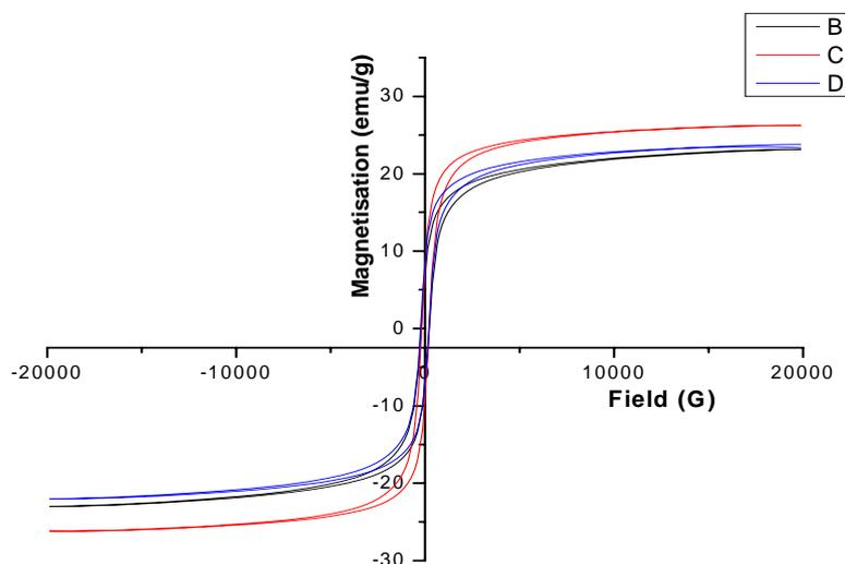
**Fig. 7.** Magnetic hysteresis curves (measured at room temperature) of  $\text{MgFe}_2\text{O}_4$  synthesised using a mixture of fuel approach and sintered at  $900^\circ\text{C}$  for 2 h: (a)  $\text{MgFe}_2\text{O}_4$ -I [using only urea ( $U/N = 2.22$ )], (b)  $\text{MgFe}_2\text{O}_4$ -II ( $0.5U + 0.5AA$ ) and (c)  $\text{MgFe}_2\text{O}_4$ -III ( $0.75U + 0.25AA$ ).
