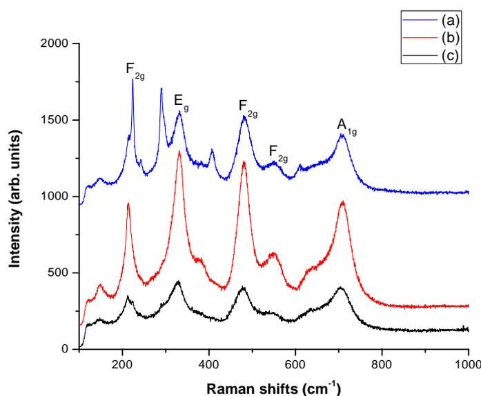
**Fig. 4.** Raman spectrum of  $\text{MgFe}_2\text{O}_4$  samples synthesised using a mixture of fuel approach and sintered at  $900^\circ\text{C}$  for 2h: (a)  $\text{MgFe}_2\text{O}_4$ -II (b)  $\text{MgFe}_2\text{O}_4$ -III (c)  $\text{MgFe}_2\text{O}_4$ -I.
