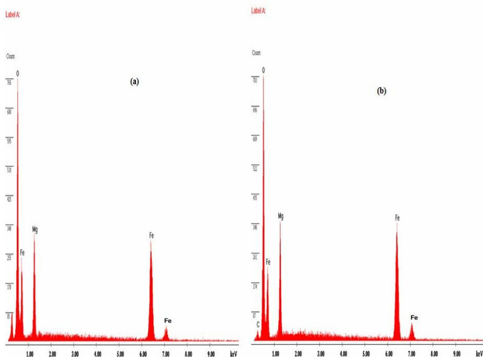
**Fig. 6.** EDAX spectra obtained using both urea and a mixture of fuel and annealed at  $900^\circ\text{C}$  for 2 h (a)  $\text{MgFe}_2\text{O}_4$ -I (b)  $\text{MgFe}_2\text{O}_4$ -II.
