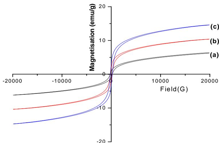
**Fig. 8.** Magnetic hysteresis curves (measured at room temperature) of  $\text{MgFe}_2\text{O}_4$  synthesised using a mixture of fuel approach and sintered at  $600^\circ\text{C}$  for 2 h: (a)  $\text{MgFe}_2\text{O}_4$ -I [using only urea ( $U/N = 2.22$ )], (b)  $\text{MgFe}_2\text{O}_4$ -II ( $0.5U + 0.5AA$ ) and (c)  $\text{MgFe}_2\text{O}_4$ -III ( $0.75U + 0.25AA$ )
