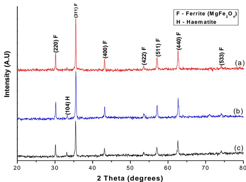
**Fig. 2.** XRD patterns of  $\text{MgFe}_2\text{O}_4$  sample annealed at  $900^\circ\text{C}$  for 2h: (a)  $\text{MgFe}_2\text{O}_4$ -II (b)  $\text{MgFe}_2\text{O}_4$ -III (c)  $\text{MgFe}_2\text{O}_4$ -I.
