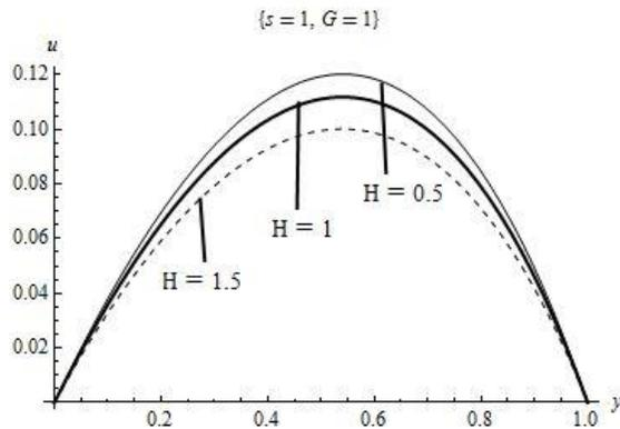
**Figure 1:** Velocity Profile for Magnetic Field Parameter.
