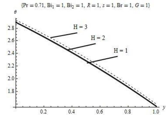
**Figure 4:** Temperature Profile for Magnetic Field Parameter.
