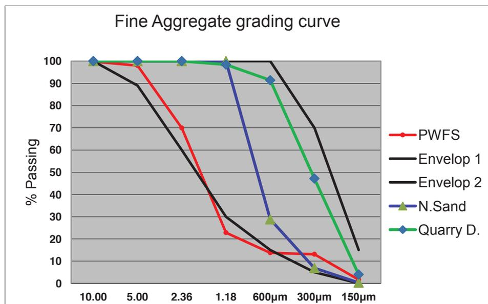
Fig. 1. Shows the Fine Aggregate grading curve
