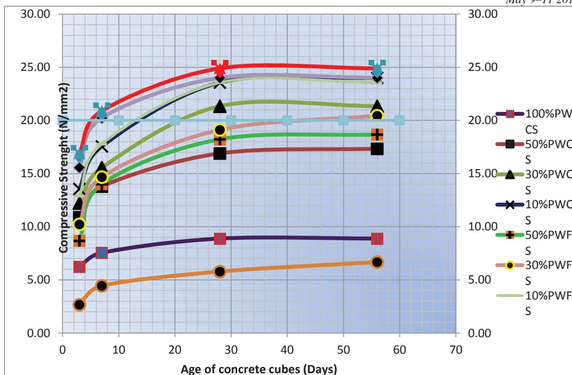
Fig. 3. Compressive Strength vs. age of concrete chart
