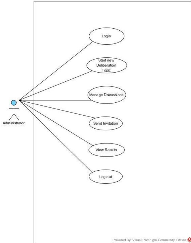
Figure 3: Use Case Diagrams of the System
