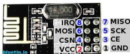
Figure 2.2: NRF24L01+ Module
